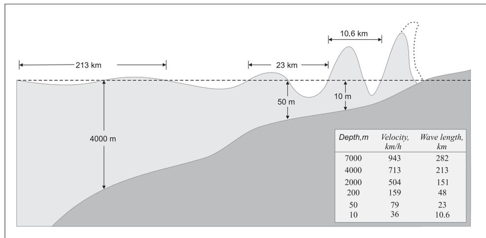
Fig 1 Shoaling effect of a tsunami<sup>1</sup>
