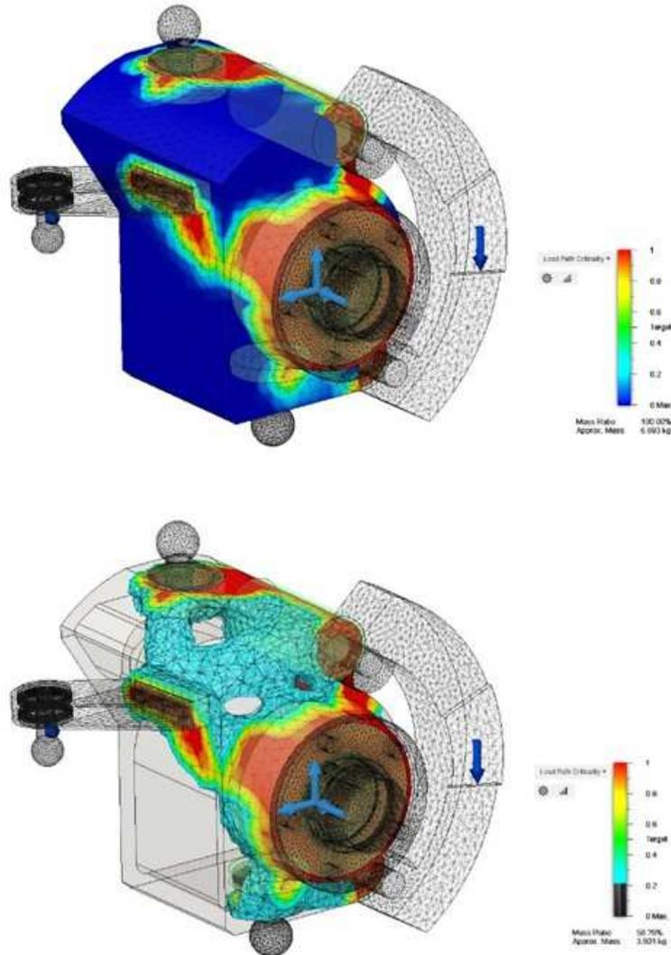
Fig. 3 - The result of topological optimization of steering knuckle
