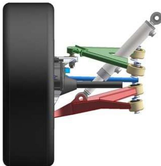
Fig. 1 - The quarter design of suspension system
