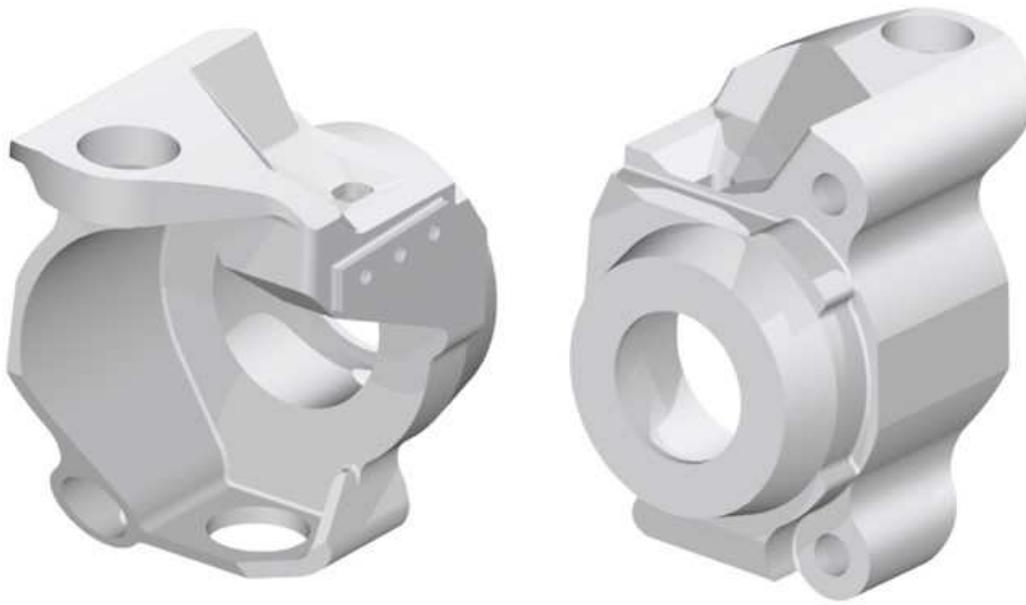
Fig. 4 - Final CAD model of steering knuckle
